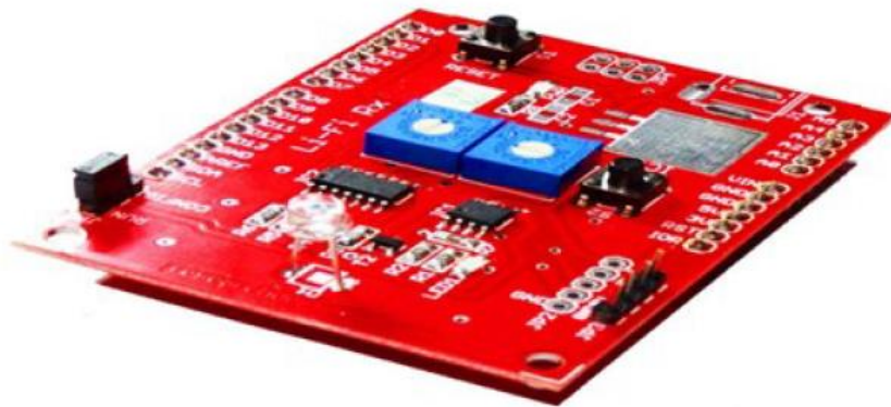
Fig 4 : Li-Fi Transmitter and Receiver Module
